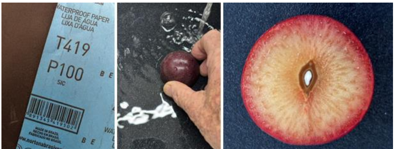
Fig. 2. (Left to right) wet and dry sandpaper is available in several grit sizes, 80015–100 grit works well. Grinding under running water prevents the paper becoming clogged. Transverse cross section of a very ripe plum.
